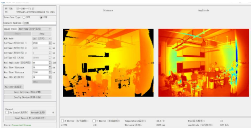
3) HDR 打开, IntTime1: 200us, IntTime1: 1200us, Min Amplitude:60 lsb, Max FPS 设置 30
